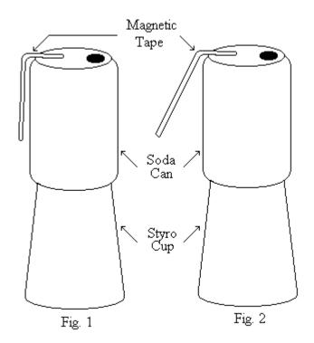
When the soda pop can is touched with a charged object, the magnetic tape will be repelled from the can and stand away from its side (fig. 2). If the can is grounded by touching the can with a finger, the magnetic tape will again fall along the can's side. The electroscope works because the magnetic tape is a conductor of electricity and not because of the tape's magnetic properties.
