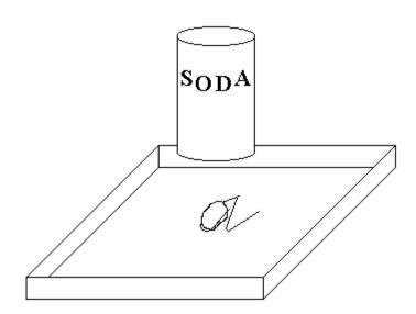
you will have to relight it). When the peanut has burned as completely as it is going to, measure the volume of water that was melted by the flame.
